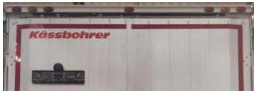
3 stop lights and 2 signal lights on the rear Door headcap
