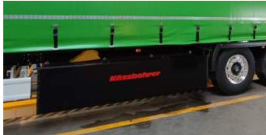
Pallet box with 30-unit pallet capacity Available for curtainsider vehicles with 5th wheel height of 1,150 mm or above
