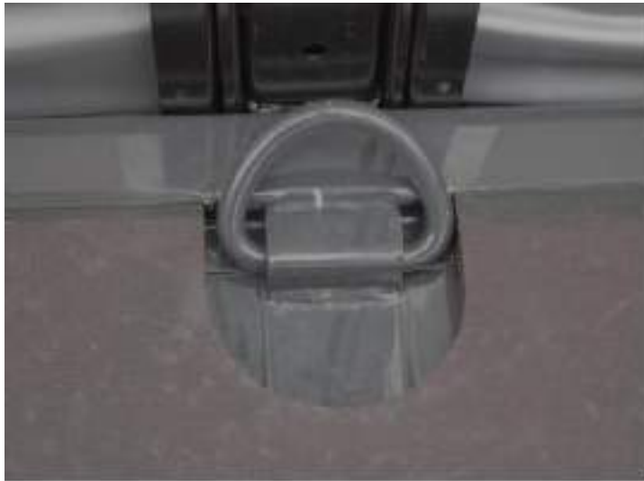
4x2 lashing rings placed on both side rails with 5-ton capacity.
