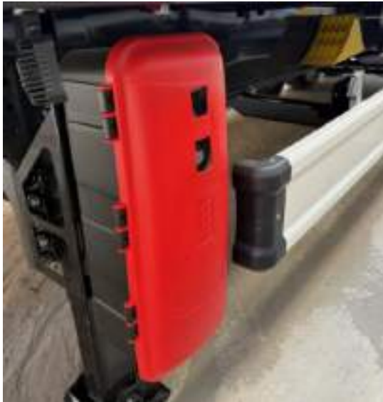
1 unit of fire extinguisher box on landing gear
