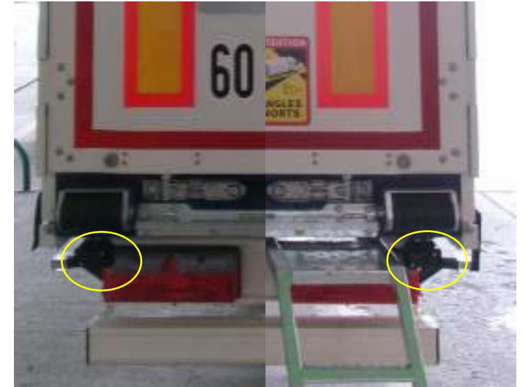
Tailguard – Rear sensor to assist with reverse maneuvers during docking using sensor guidance.
