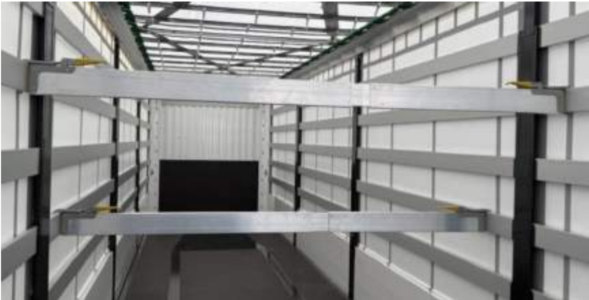
Load Stopper Bars to fix loads
