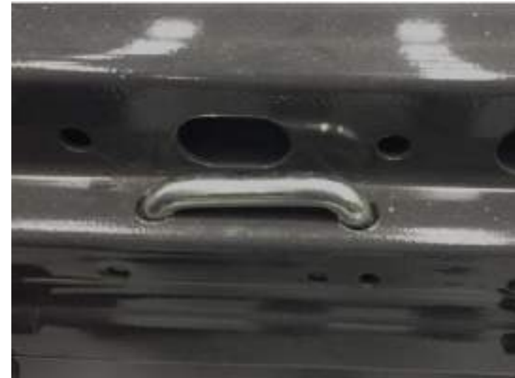
13x2 U-Type Lashing Rings with 2-ton capacity.
