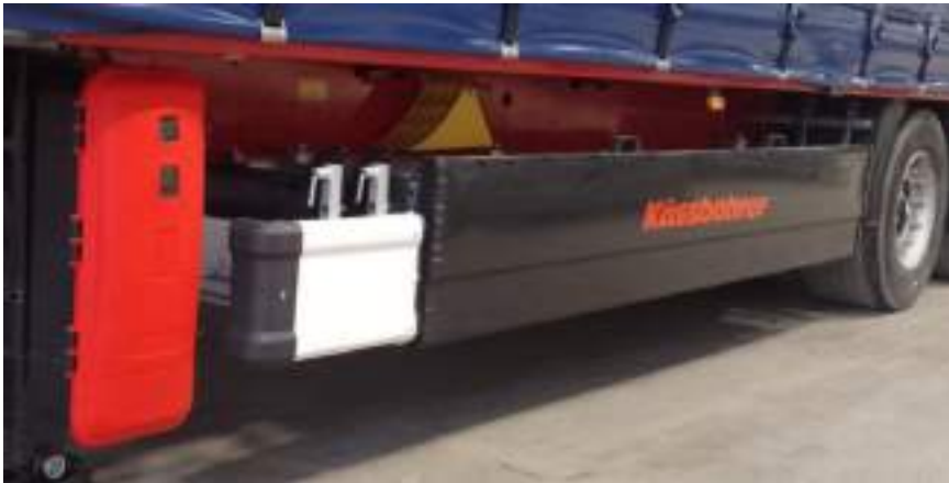
Pallet box with 24-unit pallet capacity Available for curtainsider vehicles with 5th wheel height of 1,100 mm or above
