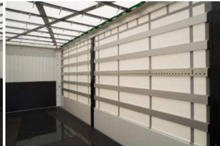
Aluminum & Steel Side Rows Steel side row has holes on it to lash spanzet.
