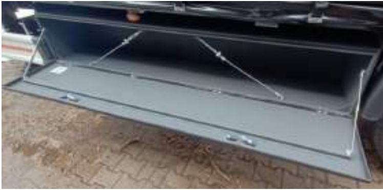
2.440 mm - PVC coated box (storage for double deck)
